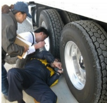
The GITI Tire Technical Center team checks tread depths at J-Mar Trucking.
